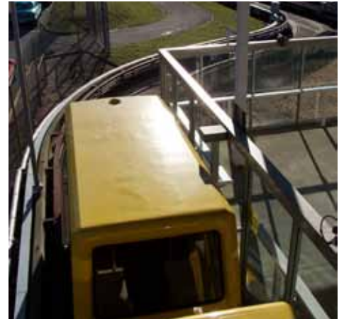
Vehicles are powered by electrified rails on one or both sides of the guideway. Vehicles steer slightly toward whichever side is powered so they can stay in firm electrical contact with the rails
