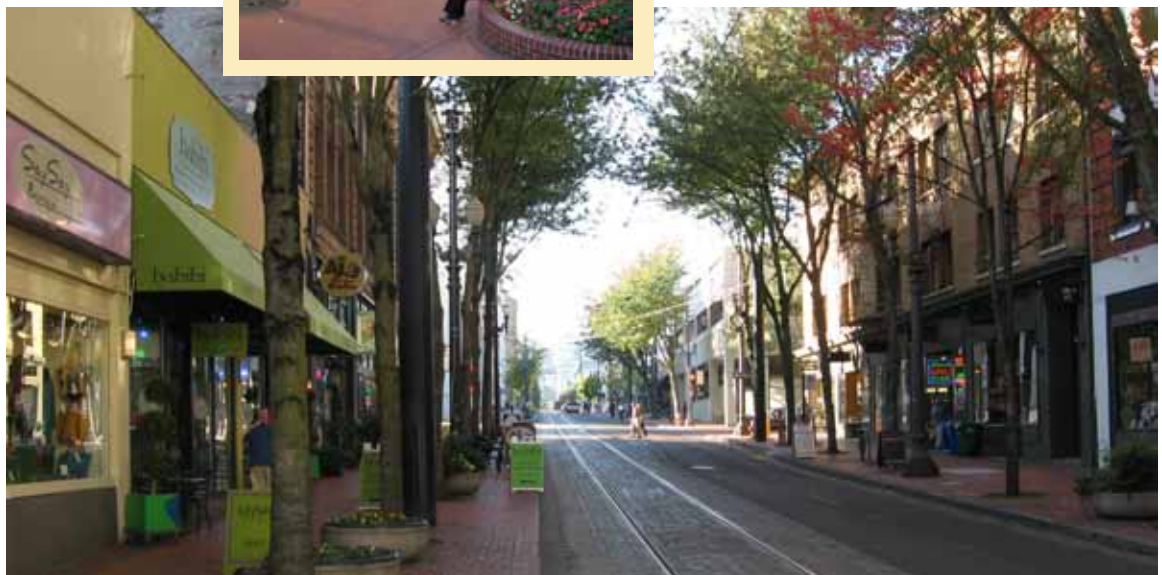
Streetcars operate in lanes shared with other traffic, eliminating the need for additional right-of-way
