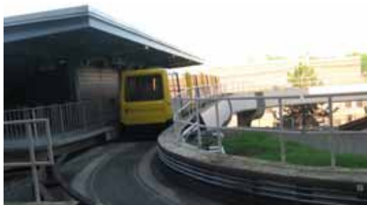
When a vehicle approaches a station, it can either continue forward and bypass the station or the wheels can turn and follow the electrified rails into the station
